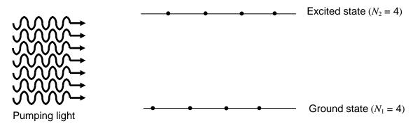
In this situation the incoming flood of photons is just as likely to cause an electron to drop (stimulated emission) as it is to cause an electron to rise (absorption). The best we can achieve here is  $N_2 = N_1$  which is not quite good enough.
