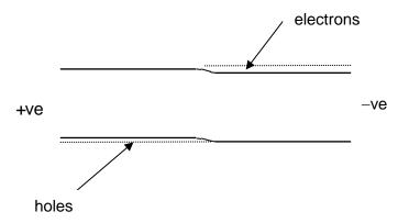
Can you see the area of population inversion? If you look carefully, there's a small region in the middle between the p-type and the n-type where we have a high concentration of electrons above holes. These are the electrons that can be stimulated to drop and provide laser light.
