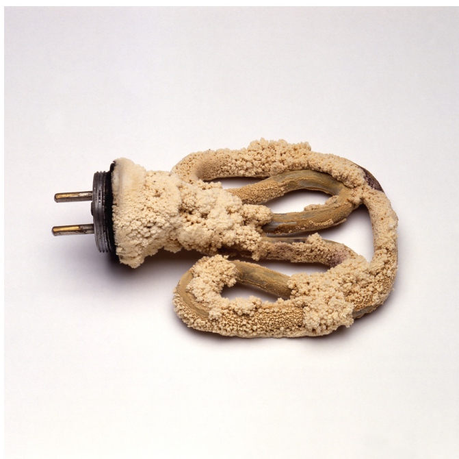
Kettle element coated with limescale John Smaller / Alamy Stock Photo
