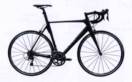
Carbon Fibre would be a good compesite meterial for use using this bites from to wake a strong and shorty materials. It is well known for being as strong as strong as strong as street but also being much lighter. This allows the cyclist to accelerate quicker and makes the bites lighter and easy to carry. Carbon Fibre can be baught in sheets and so can be shaped exity to form compuse shapes such as the bites from the strengtwith of Carbon Fibre much the cyclist.
